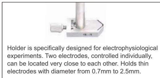
Holder is specifically designed for electrophysiological experiments. Two electrodes, controlled individually, can be located very close to each other. Holds thin electrodes with diameter from 0.7mm to 2.5mm.
