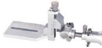
This adaptor integrates the gas anesthesia mask function while hold the rat head firmly. The adaptor can rotate the head to multi angle without blocking the anesthetic gas delivery.
