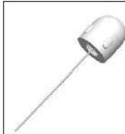
Stainless steel wire and threaded plastic cap make a dummy cannula. It can be inserted into guide cannula and fixed by screw to seal the guide cannula and prevent outflow of tissue fluid after injection. The length of the stainless steel wire can be customized.
