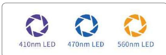
The excitation light source consists of 3 wavelengths of light (410nm,470nm,560nm), which can simultaneously record 2 ranges of excitation light (500 - 535nm, 575 - 628nm) — from the excitation of green fluorescent proteins (e.g. GCaMP) and red fluorescent proteins (e.g. RCaMP). 410nm can reflect the background noise signal.
