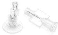
Syringe connector is composed of transparent shell and capillary tube, with a size of 25G. The front end of the injection needle can be directly inserted into the Pharmport for infusion and blood sampling, the rear end can be connected with the standard syringe.
