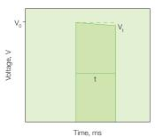
Square-wave pulse. Truncating the pulse from a capacitor after discharging it into the sample generates a square-wave pulse. The pulse length is the time the cells are subjected to the discharge. A slight drop in voltage occurs with all square-wave instruments. This drop in voltage is called the pulse droop and is measured as a percentage of the initial voltage.
