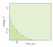
**Exponential-decay pulse.** When a capacitor charged to a voltage  $V_0$  is discharged into cells, the voltage applied to the cells decreases over time exponentially. The time required for the initial voltage to drop to  $V_0/e$  (where e is the base of the natural logarithm) is referred to as the time constant,  $\tau$ , a convenient expression of the pulse length.
