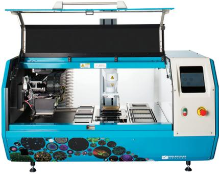
Microbial screening colony picker with sample tracking and plate handling. Fully automate synthetic biology workflows for DNA assembly, antibody discovery and protein engineering.
