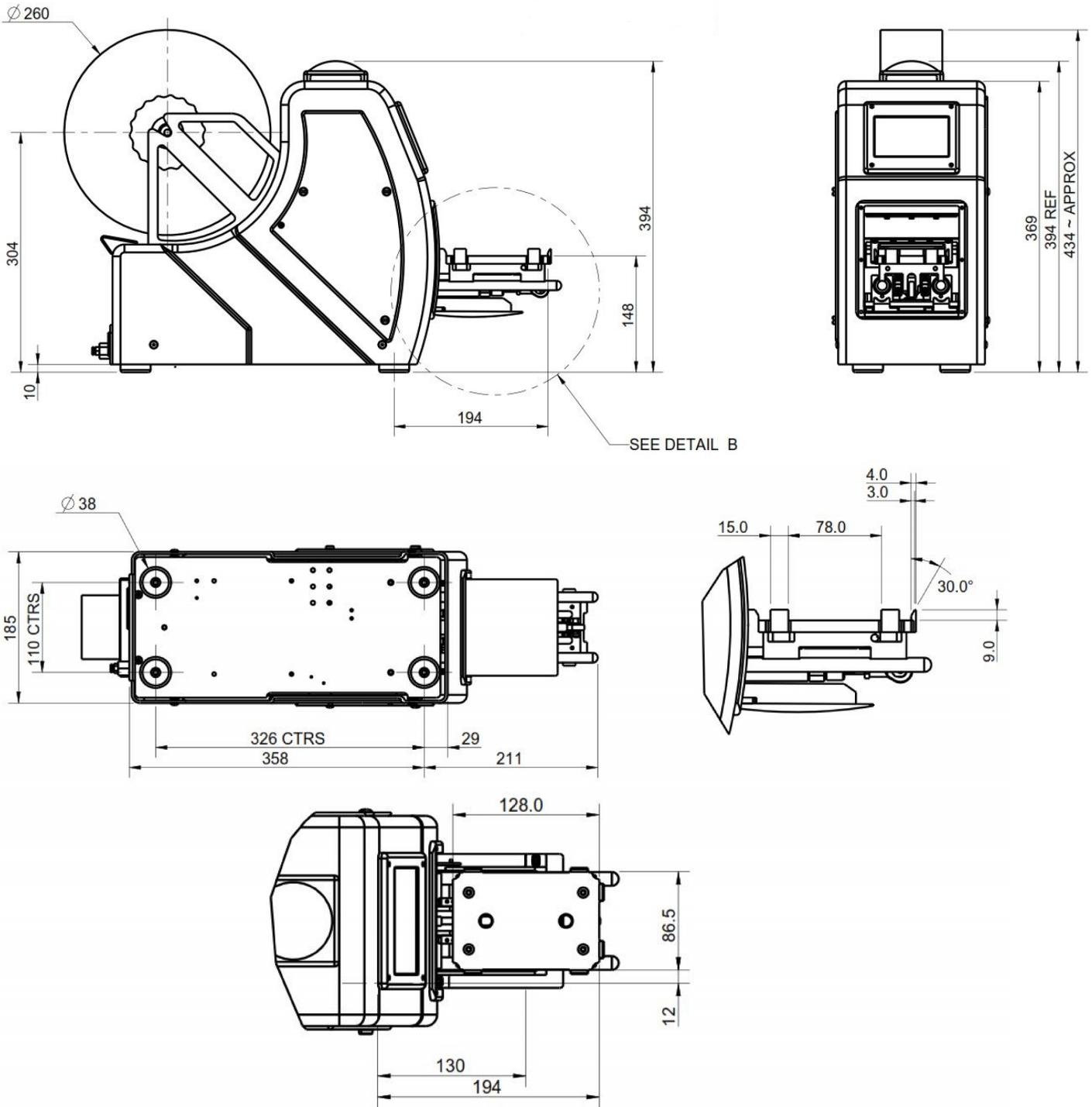
**General assembly for extended shuttle format Wasp sealer.**
