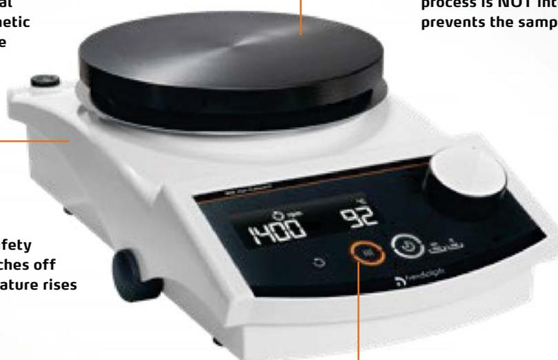
The device is switched off completely in the event of a short circuit, broken sensor of the temperature sensor and in the event of a processor fault
