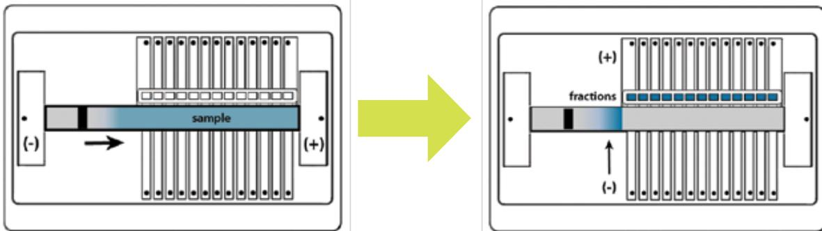
The SageELF gel cassette separates DNA along an agarose gel column. At the end of a user-programmed run time, a second set of electrodes is activated. DNA fractions are then side-eluted into 12 membrane-bound wells. The cassette design includes a novel continuous buffering system which ensures DNA does not diffuse away from the gel during separation, and that fractions are evenly collected during electro-elution.
