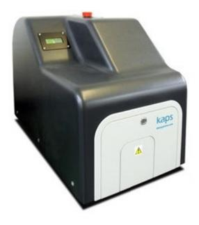
The Kaps unit is an automated adhesive pressure applied micro plate and tube rack sealer. The unit uses a roll of surface modified aluminium or plastic film approx. 78 to 85mm wide and 200m long, the roll is positioned to the rear of the sealing section via a removable stand, using a total inline method the film is pulled through the main unit, cut to between 124mm and 130mm in length and then applied to the plate top surface to create the seal between plate and film.
