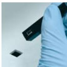
**1.** Position the TrayCell inside the cell holder of the spectrophotometer.
