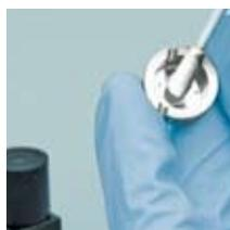
**5.** Clean the measuring window and the cap (the TrayCell remains in the spectrophotometer).
