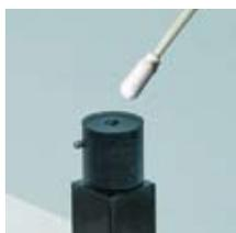
**4.** Take off cap, retrieve sample with a pipette, if desired.
