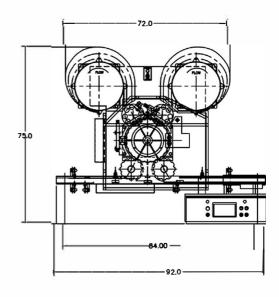
Approximate Dimensions W x D x H (Set up) 92" x 75" x 50" (2338mm x 1905mm x 1270mm) (does not include enclosure) Approximate Dimensions W x D x H (Crated) 113" x 82" x 58" (2870mm x 2082mm x 1473mm) Approximate Weight (Net) 3500 lbs. (159kg.)Approximate Weight (Gross) 4500 lbs. (2045kg.)
