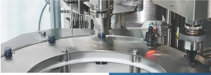
The RFPC is PLC controlled and features a stainless steel exterior and all liquid contact parts of 316L stainless steel. It has a raised sanitary conveyor that transports containers to and from the filling/plugging/capping area and comes with a no plug/no cap detection system. Optional features include servo driven torque heads, over/under torque container rejects system, statistical torque value reporting, no plug/no cap reject system and make up/back up detection systems.
