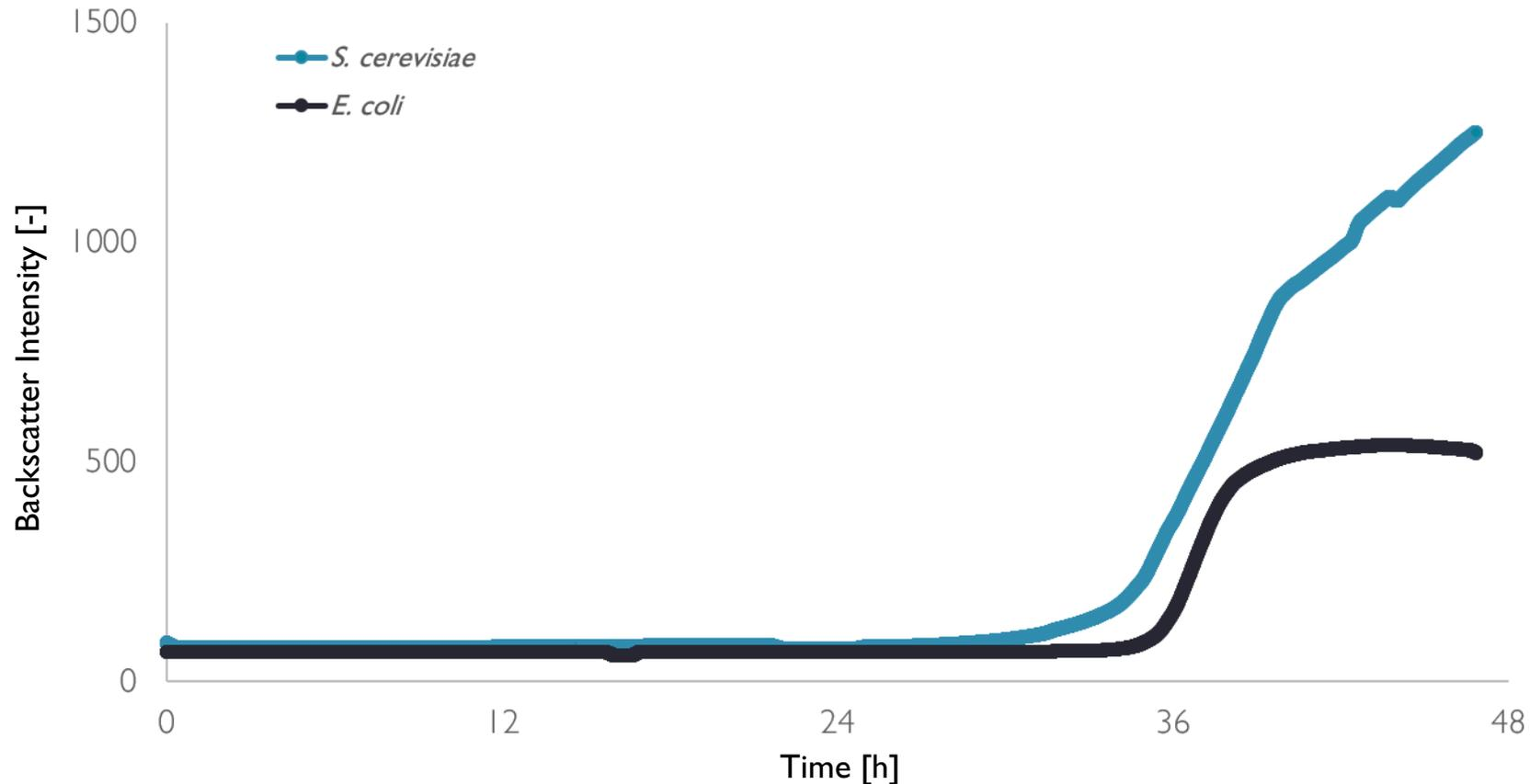
The first LIS cartridge was filled with an *E. coli* culture (LB medium + Kanamycin, OD600 = 0.1). 1 ml of this culture was dispensed into a 250 ml shake flask filled with 25 ml LB + Kanamycin using a single shot after an initial delay of 32 h. The second cartridge was filled with a *S. cerevisiae* culture (YPD medium + 0.5 M NaCl, OD600 = 0.1). 1 ml of that culture was fed into a 250 ml shake flask filled with 25 ml YPD medium + 0.5 M NaCl using the same feeding profile.
