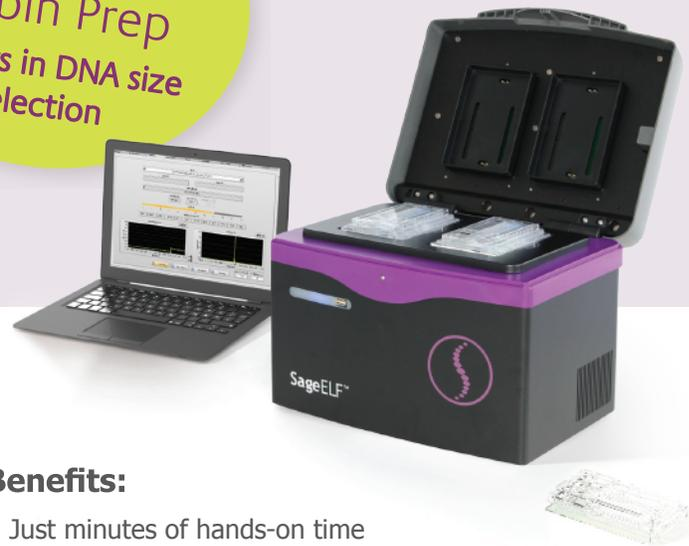
The SageELF gel cassette separates proteins along an agarose gel column, at the end of a user-programmed run time. As a second set of electrodes are activated, fractions are side-eluted into 12 membrane-bound wells. The cassette design includes a novel continuous buffering system which ensures the proteins do not diffuse away from the gel during separation, and that fractions are evenly collected during electro-elution.
