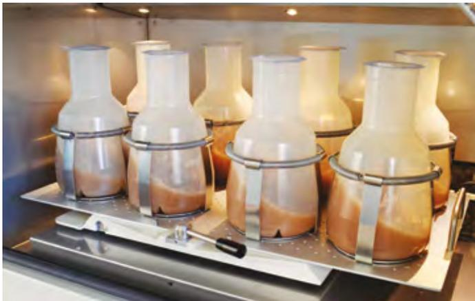
To create a seed culture, grow up 50mL of the microbe of choice in a 250mL Ultra Yield® Flask with Enhanced AirOtop™ Seal: 50mL working volume. The overnight culture should be grown for at least 16 hours, at a temperature of 37°C at 350rpm (25mm or 1" Throw). This should be done in an orbital shaker using flask clamps. The 50mL working volume will then seed a 2.5L Ultra Yield® Flasks. Please note that 1:5000 of anti-foam should be used for limiting foaming of the culture.
