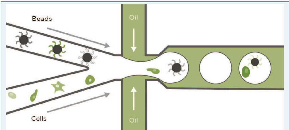
**Figure 1 Schematic of the encapsulation of barcoded mRNA capture beads with single cells.** Tens of thousands of single cells are co-encapsulated with uniquely barcoded beads. The cells are lysed inside the droplets and their mRNA content is captured by the beads. These beads are subsequently recovered and processed for downstream analysis using NGS-technologies.
