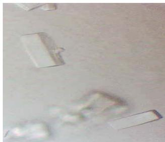
**Figure 5.** Crystals of an unknown protein (1139) grown by the sitting drop vapor diffusion method using CrystalEX microplates.
