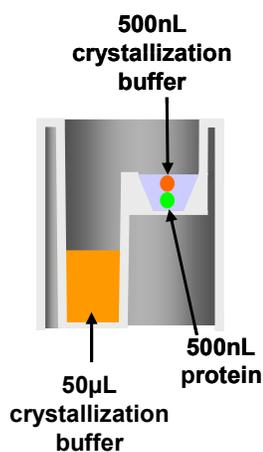
**Figure 3.** Crystallization by sitting drop vapor diffusion technology in a well from the 96 well CrystalEX microplate
