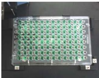
**Figure 4.** The 96 different crystallization buffers are simultaneously dispensed into the 96 well CrystalEX microplate using the Hydra system while the protein is dispensed with the NanoFill dispenser.
