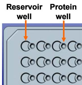
**Figure 2.** Each CrystalEX crystallization microplate has 96-round buffer reservoir wells and 96 conical flat bottom protein wells.
