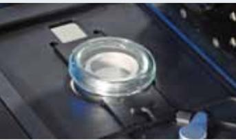
The isolation and enrichment of individual live cells for culture and differentiation experiments or for their proteomic and genomic analysis is of increasing interest in stem cell research, cancer research and tissue engineering. The mmi CellCut Plus in combination with the newly developed mmi LiveCellChamber enables contamination-free isolation of live cells in living culture.
