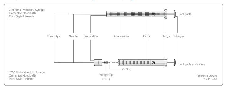
Microliter syringes have a stainless steel plunger which is individually hand-fitted to its matching glass barrel. The hand-fitting process is finely controlled to create a liquid-tight seal between the barrel and the plunger. Plungers for Microliter syringes cannot be interchanged or replaced if damaged.
