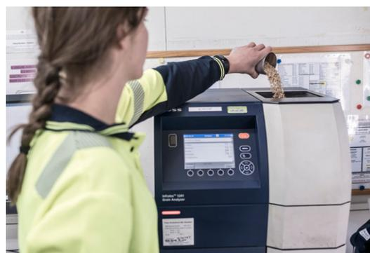
The Infratec™ 1241 is a whole grain analyser using near-infrared transmittance technology to test multiple parameters such as moisture, protein, oil, starch etc. in a broad range of grain and oilseed commodities.
