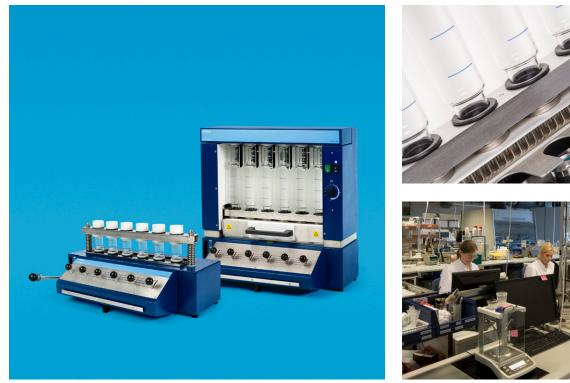
The FT 122 Fibertec<sup>™</sup> Hot Extraction Unit, for hot hydrolysis and extraction with built-in systems for heating and filtration, performs fibre analysis according to Weende, van Soest and other recognised methods, using externally preheated reagents.
