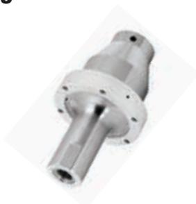
Booster horns increase the intensity of standard 3/4" and 1" horns. Boosters attach between the converter and horn to increase amplitude by the gain ratio indicated below.
