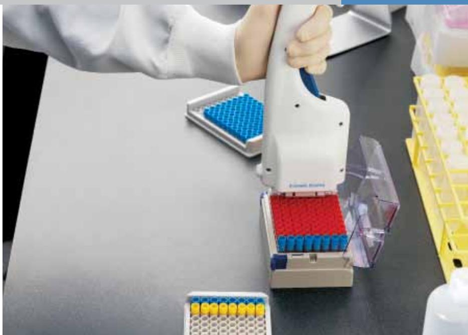
**Increase Efficiency.** The Thermo Scientific 8-Channel Decapper speeds the processing of laboratory samples. Fill uncapped tubes, then cap eight tubes at once with caps from Thermo Scientific ScrewTop Cap trays. Or uncap, fill and recap tubes with the same caps or new caps.
