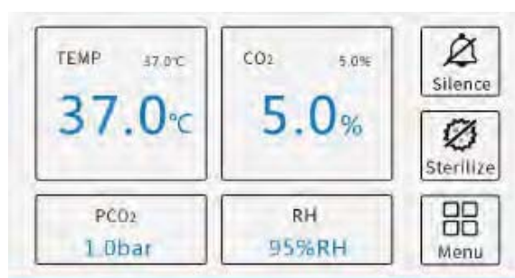
Real-time display of carbon dioxide concentration, temperature and humidity
