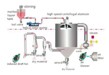
This evaporation process removes heat quickly so that the product is dried gently without being affected by heat. The product becomes powder, particle, or lump within seconds.
