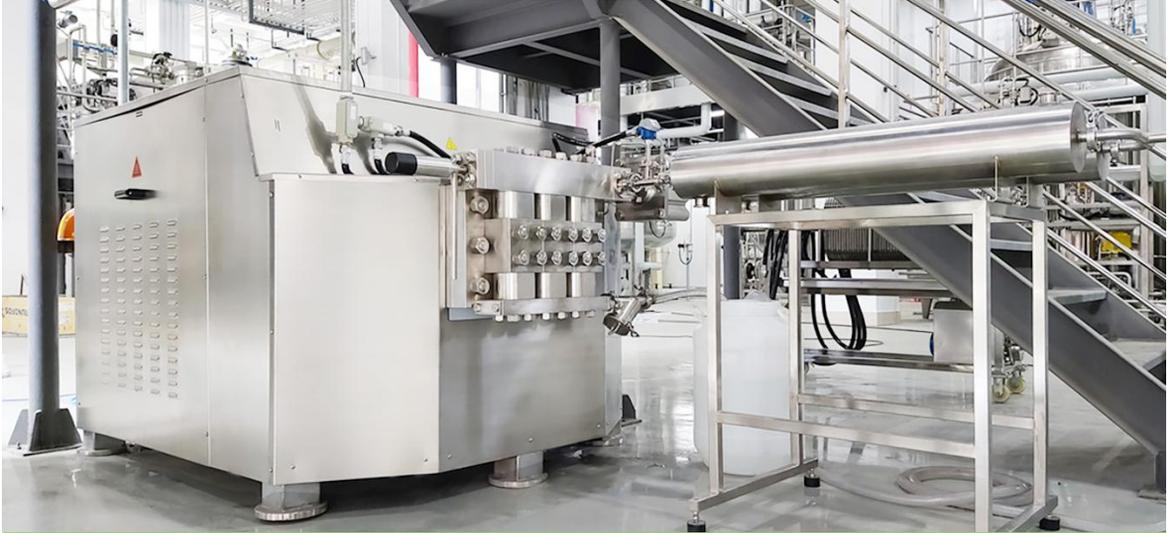
2000L cell wall breaking high pressure homogenization system
