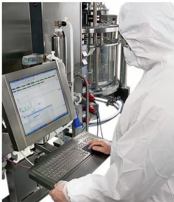
Fig 3. Intelligent Packing greatly simplifies the packing of AxiChrom columns used with ÄKTA™ systems.
