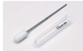
Homogeniser as centrifuge tube with teflon pestle, cylindrical
