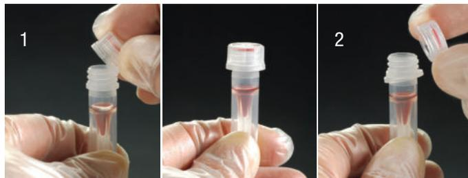
1. Screw cap until locking ring clicks over serrated tube neck.
