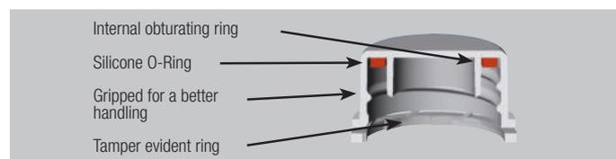
Withstand centrifugation at **17.000 xg**.
