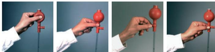
1. Evacuate the air by pressing the bulb, as the drawing indicates
