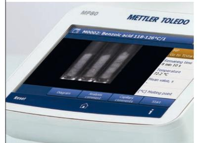
Measurement results can be influenced by the operator. Save time and money and reduce operator training and influence with fully automatic determination of melting, boiling, slip melting, and cloud points.
