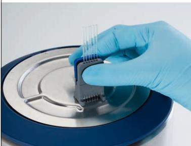
In today's fast-paced environment, high throughput processing is essential. With the Excellence Melting Point System, you can run up to six samples simultaneously, saving you valuable time and effort.
