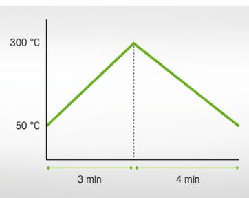
METTLER TOLEDO's Excellence Melting Point Systems are always ready to go. Program the instrument to return to a pre-specified temperature after the experiment. Rapid heating and cooling cycles mean that you can complete more analyses in a short amount of time.
