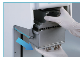
Pull out the pipetting head
