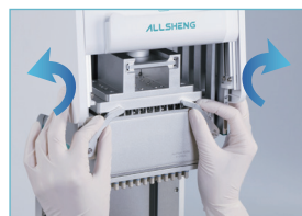
Release the handles on both sides
