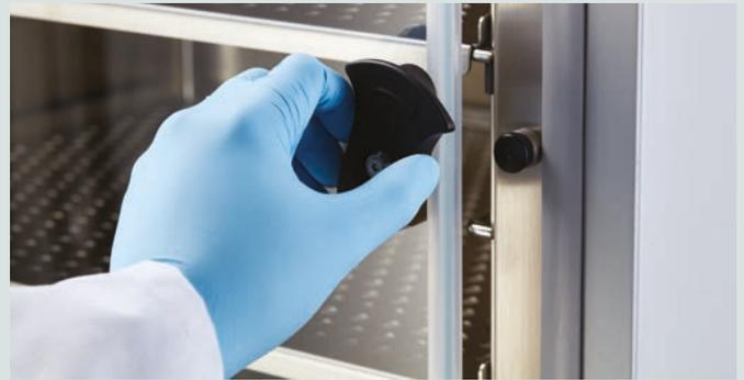
The tightly closing inner door latches also utilize the new magnetic closure concept. The dual direction latch on the inner door of the C170i can be simply pulled or turned to open, then pushed or turned to close. This way, the CellXpert C170i CO<sub>2</sub> Incubator can provide both advanced vibration protection for sensitive cells and adjust to differing user habits.
