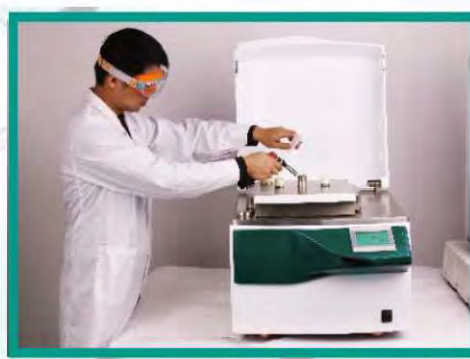
Sterilize the sample port with a flame gun
