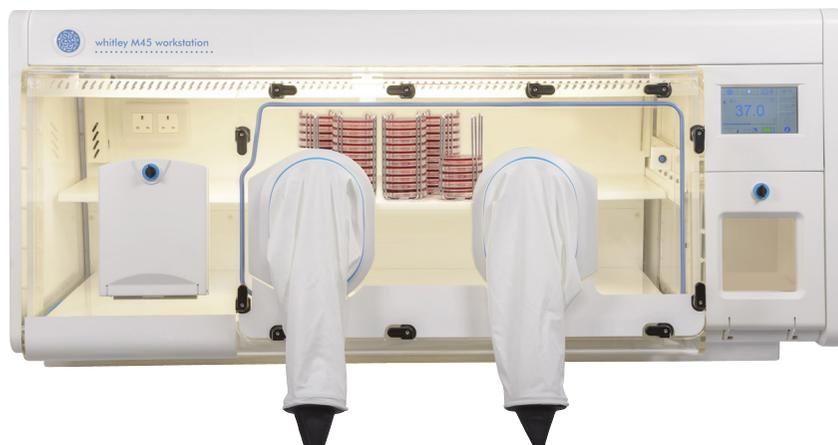
The M45 has three ports for convenient user access to the entire incubation and working areas. This workstation can accommodate over 780 x 90mm Petri dishes whilst still providing a generous working area. The M45 is used in the study and isolation of fastidious anaerobes such as *Campylobacter* spp. and *Helicobacter pylori*.
