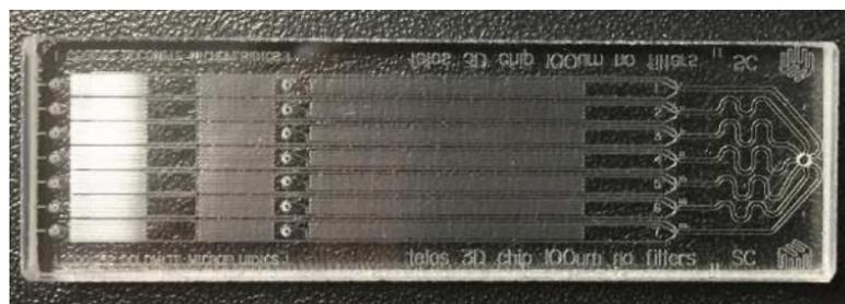
Figure 3 Telos 1 Reagent 3D Flow Focusing Chip SC 100  $\mu\text{m}$
