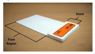
The  $iBind^{^{TM}}$  Card is placed on the  $iBind^{^{TM}}$  Western Device so that it is aligned with the stoppers and alignment tabs.
