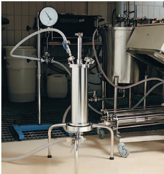
**Fig 2.** The FineLINE column is easy to pack and operate to the high standards of hygiene applied in the production of biopharmaceuticals.
