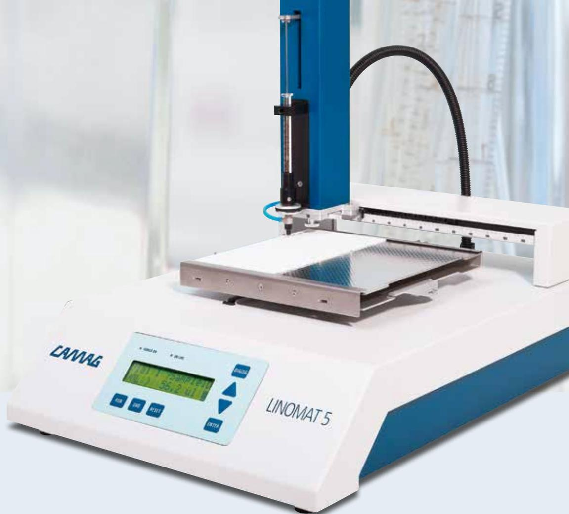
With the Linomat 5 samples are sprayed onto TLC/HPTLC plates with nitrogen or compressed air. Sample application is automatic, only changing the syringe (filling, inserting and rinsing) is manual. The Linomat is suitable for routine use.
