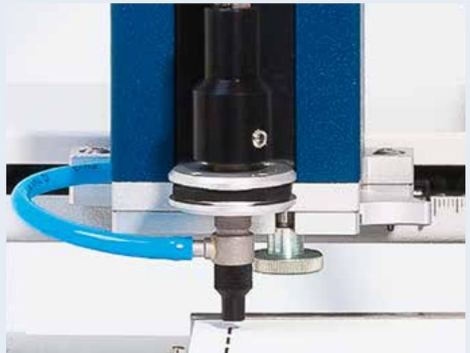
*The combination of the special dosage syringe with the spray nozzle of the Linomat 5 ensures the focused spraying-on of samples on very small areas.*
